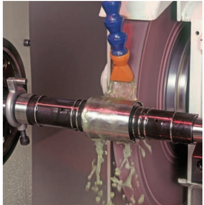
94AB BAS – Advanced grain technology used in Cylindrical and Centerless applications. This grain can be used to grind steels in either soft or hard state.
